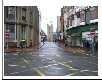
A northbound contra-flow from Kings Road could be introduced – current width 4.5m. Or a cycle only track on western footway
