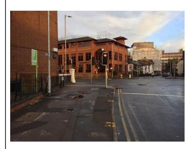
The Diag 955 cycles only sign is wrongly angled so that it is not clearly visible from Gt Knollys St. A Diag 954.4 Except Cycles plate could usefully be added below the left of the two No-entry signs for clarity.
