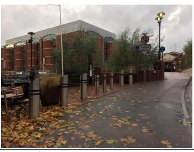
There is inadequate shared-use signing by Yield Hall Lane. The Diag 956 shared-use sign should be located on the post by the Oracle path and angled correctly to indicate the Oracle path not Yield Hall Lane. The cycle direction signs are hidden behind the other road-sign. A new cycle signing post near the picture foreground would help clarify the cycling routes.
