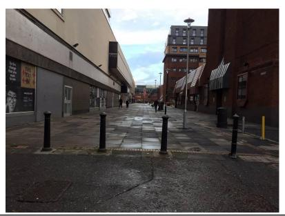
No signing in Queens Place from Oxford Road and Hosier Street to show cycling allowed. Diag 956 shared-use signs should be fitted to some end bollards and lighting columns.
