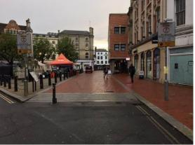
The existing southbound signs to diag 618.3 is wrong in that it includes "No vehicles", this is only allowed where all vehicles are banned. Sign should be changed to remove 'No Vehicles' by replacing with the new Diag 618C 'Pedestrian and Cycle Route' sign.
