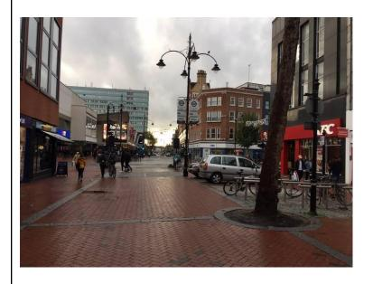
There is no signage to show when cyclists could remount. Diag 618.3C 'Pedestrian and Cycle Zone' signs could be used on the backs of the two existing no cycling signing.
