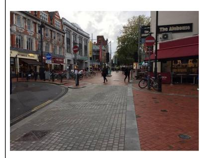
Cycling is permitted but the no entry signing is confusing. The No-entry sign on the right probably refers to the Butter Market so should be angled outwards further. Maybe it should also have an additional Diag 954.4 'Except Cycles' plate added below. The Buses only sign to the left would be better located further left as it appears to refer to Broad Street. Alternatively, the new Diag 618.3C 'Pedestrian and Cycle Zone' sign could be used to replace the No-entry.
