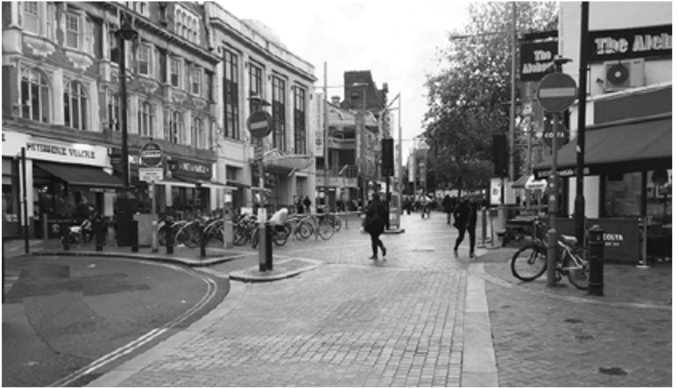
Broad Street East - the no-entry signs seem to contradict the unsigned cycle gap. Again, a Diag 618.3C sign is needed.
