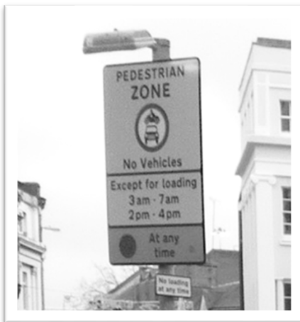
Market Place - the wrong sign is used on the west side prohibiting cyclists from using the route. Again, change signage to the Diag 618.3C
